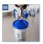
Pull the spray gun upwards to disconnect cup from the spray gun.
