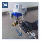
Disconnect air line. Invert gun and pull trigger to release excess paint.
