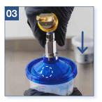
Select the right adapter, align the spray gun with the arrow and push down until firmly in place.
